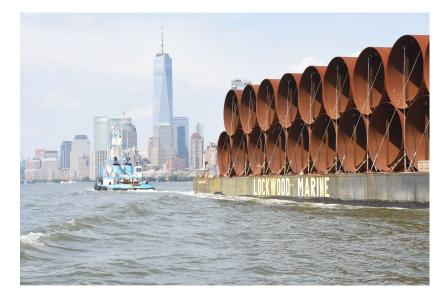
Steel liners for the Delaware Aqueduct Bypass Tunnel with Freedom Tower in background
